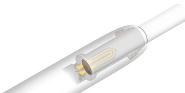
Figure 2. Illustration of the tobacco stick insertion into the heating system of the first iQOS devices
